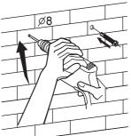
Drill holes using a 8mm dril bit (not supplied) and insert wall plugs. (Note: Before drilling always check for pipes ad cables)
